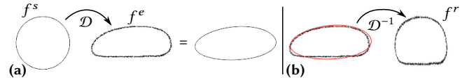
Fig. 5. Deformation analysis — (a) The parametric deformation \mathcal{D} is estimated using as-rigid-as-possible registration between the source f^s and exemplar f^e frames. (b) The residual frame f^r is then computed by applying the inverse deformation \mathcal{D}^{-1} on f^e .
