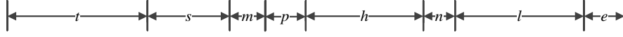
Fig 2. HTTP log structure, where t is the timestamp, s is source IP, m is method, h is hostname, p is protocol, n is port, l is path and e is web page's file type.
