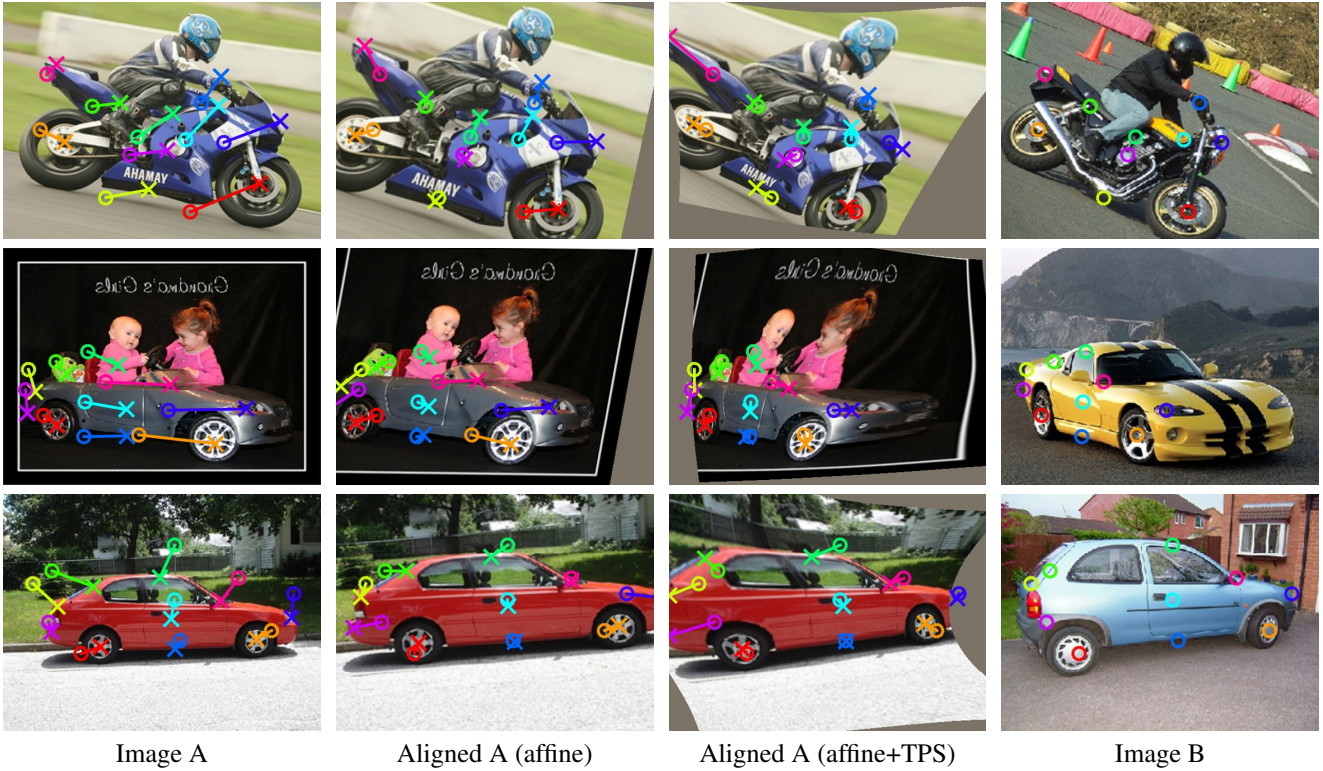
Figure 11: Example image pairs from the Proposal Flow dataset demonstrating changes in viewpoint. While the affine stage can correct for the size and orientation of the object, the thin-plate spline stage is able to perform a non-rigid deformation which can, to some extent, compensate for the change in viewpoint.
