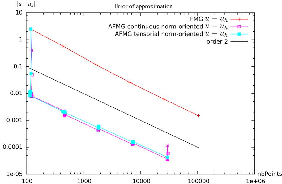
Figure 5: 2D boundary layer test case, norm-oriented methods: approximation error convergence in terms of number of vertices.
