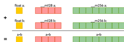
FIGURE 3: Summation example of single precision floating-point values using : (■) scalar standard C++ code, (■) SSE SIMD-vector of 4 values , (■) AVX SIMD-vector of 8 values.
