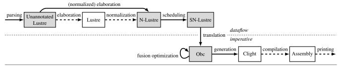
**Figure 1.** Clock-directed modular compiler architecture: the gray boxes and the solid arrows are addressed in this paper. The white boxes and the dashed arrows are addressed in previous work [2, 3] or by CompCert [40].
