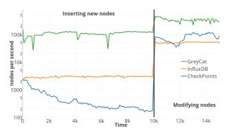
Fig. 3. Write throughput when creating and updating nodes
