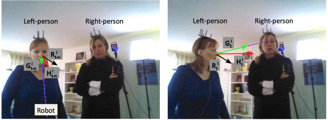
Figure 1. This figure illustrates the principle of our method and displays the observed and latent variables associated with a person ( left-person indexed by i ). The two images were grabbed with a camera mounted onto the head of a robot and they correspond to frames t - n (left image) and t (right image), respectively. The following variables are displayed: head orientation (red arrow), \mathbf{H}_{t-n}^i, \mathbf{H}_t^i (observed variables), as well as the latent variables estimated with the proposed method, namely gaze direction (green arrow), \mathbf{G}_{t-n}^i, \mathbf{G}_t^i , VFOA, \mathbf{V}_{t-n}^i, \mathbf{V}_t^i , and head reference orientation (black arrow), \mathbf{R}_{t-n}^i, \mathbf{R}_t^i (that coincides with upper-body orientation). In this example left-person gazes towards the robot at t - n , then turns her head to eventually gaze towards right-person at t , hence her VFOA switches from \mathbf{V}_{t-n}^i = \text{robot} to \mathbf{V}_t^i = \text{right-person} .
