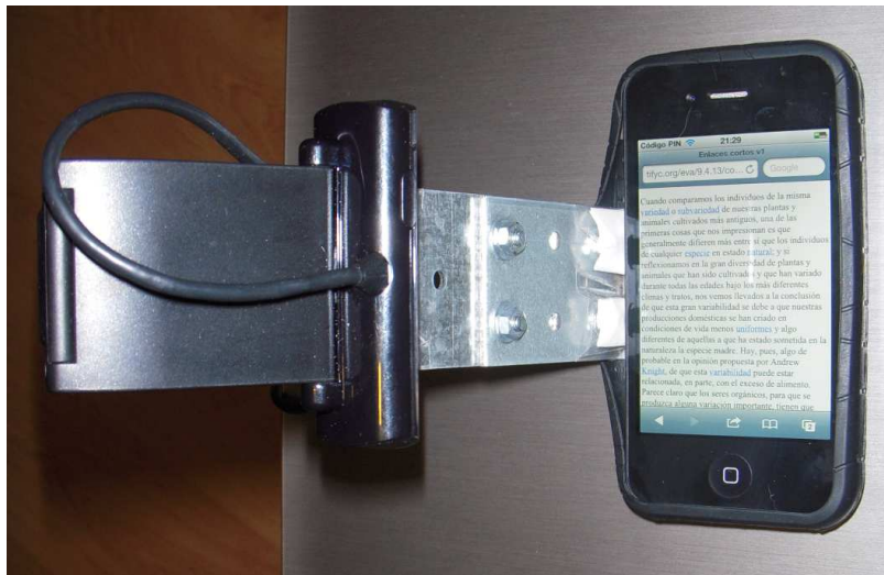
Fig. 2. Mechanism used to record user interactions.
