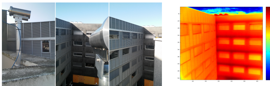
Figure 16: Inria test bed, and main IR image around sunrise.
