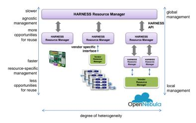
Figure 2: A heterogeneous cloud computing platform, supporting various types of resources, can be built by composing resource managers that implement the HARNESS API in a hierarchical system.
