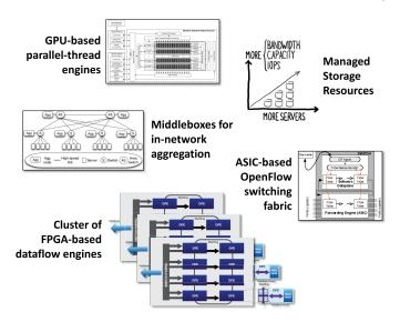
Figure 1: The HARNESS resource set consists of a group of compute, communication and storage resources. Some of these resources include (clockwise from top): (a) GPU accelerators, (b) managed storage volumes with performance guarantees, (c) hybrid switches that can handle millions of access control rules, (d) a cluster of FPGA-based devices that can be accessed via network, and (e) general-purpose middleboxes that allow application-specific network functions to be performed along network paths.
