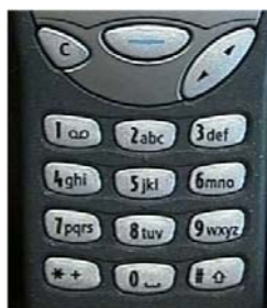
Figure 1. The keypad layout on a Nokia 3210.
