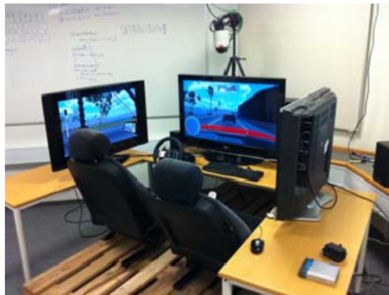
Figure 3. The physical setup of the simulator.
