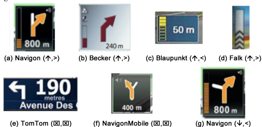
Figure 3. Design of spatial approach in different navigation systems. Legend: ‘↑’=Upwards; ‘↓’=Downwards; ‘>’=Increasing; ‘<’=Decreasing, ‘☒’=Feature not present
