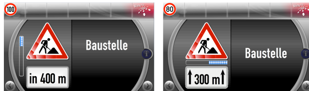
Figure 5. Two screenshots of displays for the road works use-case. Distance is indicated in numerical form (in 400m/ 300m) accompanied by a graphical bar representing relative spatial information. The left side depicts a screenshot for approaching road works and the right side shows a presentation while driving within a road works section.
