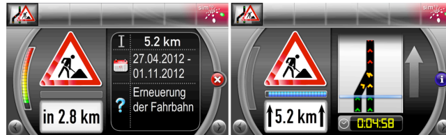
Figure 14. Official sim TD screenshots of road works information containing a color-coded approach bar (left) and a single-colored horizontal progress bar (right).
