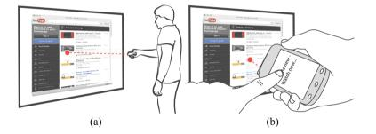
Fig. 8. Using the mobile phone as a remote control for browsing web pages on a TV set.
