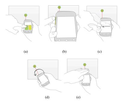
Fig. 2. Basic selection and input options supported through PointerPhone: (a) software buttons;(b) hardware buttons; (c) touch-based gestures; (d) rotation-based interaction; and (e) proximity activation.
