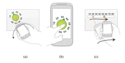
**Fig. 3.** Controlling widgets for entering data can be implemented in three ways: (a) Rotating the phone to change the value; (b) manipulating the proximal widget representation on the phone screen; (c) distal interaction with widgets on the remote screen.
