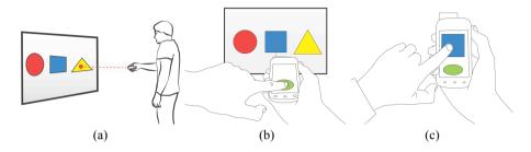
**Fig. 1.** Using the mobile phone as a pointing device enables versatile interactions with remote screens: (a) Pointing to targets. (b) Performing actions on the personal phone such as selecting and downloading an item. (c) Further interaction with data on the phone.
