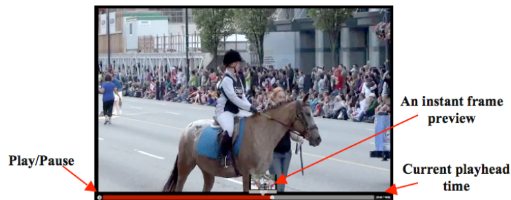
Figure 2. The video player component contains play/pause button, video seek-bar, and a pop-up thumbnail shown when the pointer is over the time bar.
