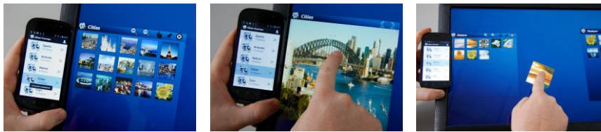
Fig. 4. The photo sharing application: (left) extended overview; (middle) focus on a single image; (right) sharing images with another user by dragging an image from one extended interface to another.
