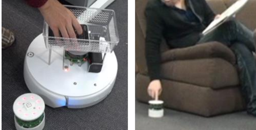
Fig. 6. Two Ways to Specify a Goal. The user can specify a goal of the robot by pressing a button on the remote control attached to the robot (left). The user can also specify a goal by pressing the button of the pebble (right).
