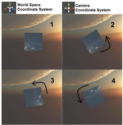
**Fig. 3.** For all frames the world space and camera coordinate systems are shown at the top of this illustration. The user is always looking down the *z-axis*. Frames 1 through 4 illustrate rotating a cube along the view direction (i.e. the *z-axis*). We can clearly see that only the camera coordinate system influences the rotation of the object.
