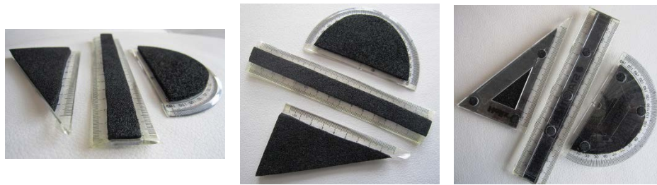
Fig. 3. Final tangible drawing tools (conductive foam)
