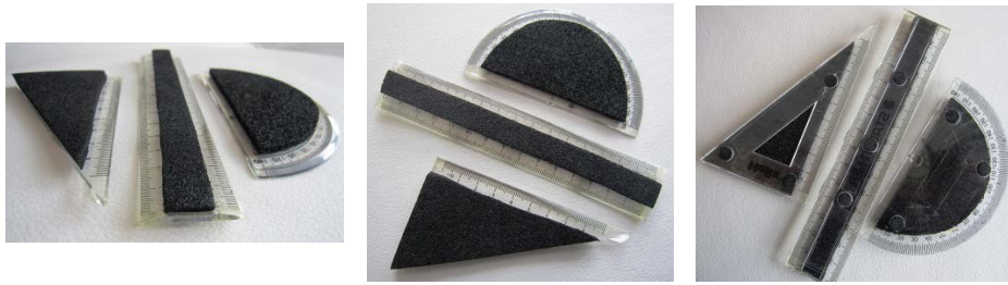
Fig. 3. Final tangible drawing tools (conductive foam)
