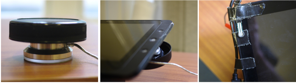
Figure 2: Hardware setup for our study: Griffin Technologies PowerMate with extended radius (right), the dial affixed to the rear of the tablet (centre) and the pressure sensor affixed to the top-left of the bezel of the tablet (left).
