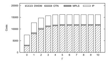
Fig. 2. CAPEX costs versus  $\Gamma$  uncertainty parameter for the Géant network with variable configuration
