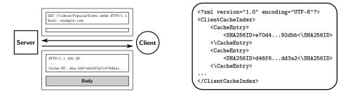
Fig. 1. HTTP header field extension
