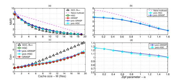
Fig. 5. Comparison of the total minimum rate normalized by the 1-user network minimum rate with respect to : a) the cache size with  $\alpha = 0$ , and b) the Zipf  $\alpha$  parameter with M = 2 files, and the gain of the coded over the uncoded scheme with respect to: c) the cache size with  $\alpha = 0$ , and d) the Zipf  $\alpha$  parameter with M = 2 files.
