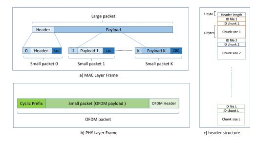
Fig. 3. An example of the proposed frame structure.
