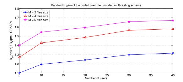
Fig. 6. The bandwidth gain of coded multicasting over naive multicasting for different memory cache sizes.
