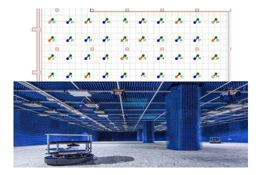
Fig. 4. CorteXlab platform and the nodes placement map.
