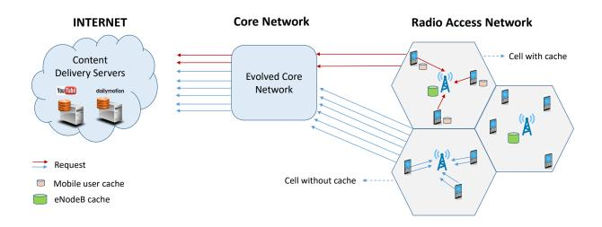
Fig. 1. Caching within the radio access network: impact on network load and traffic congestion.
