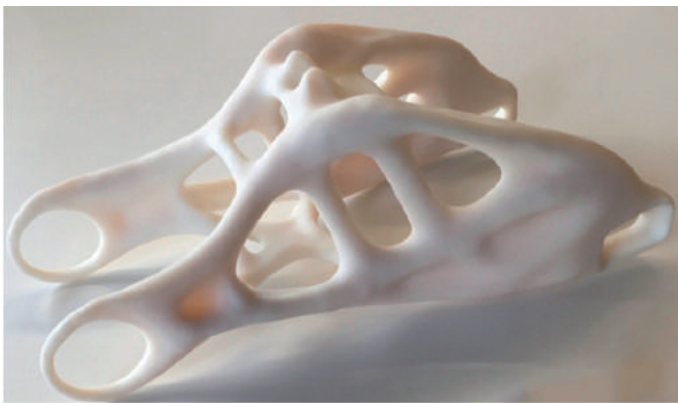
Figure 82: An early, bone-like, prototype of the Lightning Motorcycle swingarm. Autodesk's Dreamcatcher software can craft a swingarm – the piece that hinges the rear wheel to the bike's frame – by starting with weight and strength as the beginning design elements, rather than a predetermined shape of metal.
