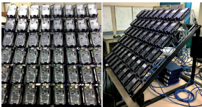
Figure 72: IBM TrueNorth system, able to simulate 48 millions of artificial Neurons Source: IBM
