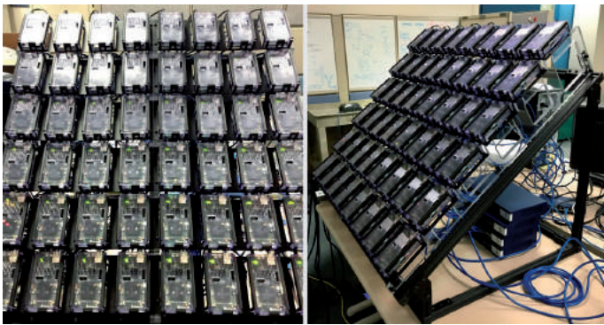
Figure 72: IBM TrueNorth system, able to simulate 48 millions of artificial Neurons Source: IBM
