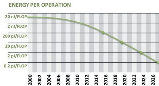
Figure 55: Evolution of energy per floating point operation Source: www.top500.org
