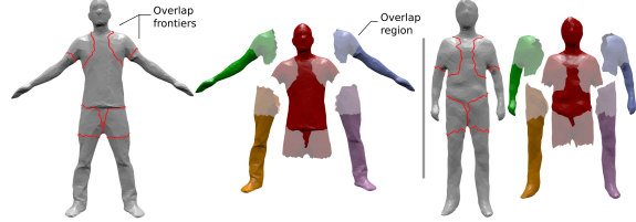
Figure 2: Body parts: shaded colors represent overlapping regions between parts delimited by user given curves.
