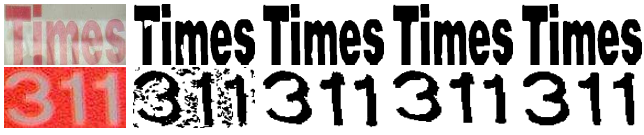
Fig. 6. Illustration of binarization results with different number of iterations of graph cut. Here, we show the original image and the results with 1, 3, 5 and 8 iterations (from left to right).
