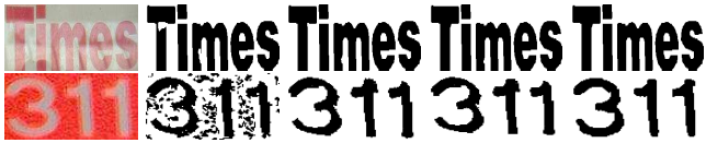
Fig. 6. Illustration of binarization results with different number of iterations of graph cut. Here, we show the original image and the results with 1, 3, 5 and 8 iterations (from left to right).
