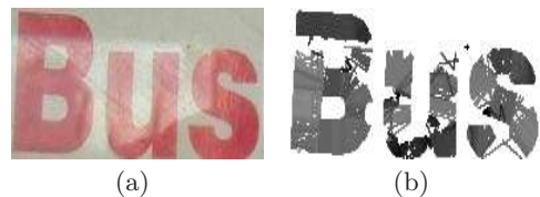
Fig. 4. (a) Input image. (b) Character-like strokes obtained using the method presented in Section 5. Darker regions in (b) represent parts with lower stroke width.
