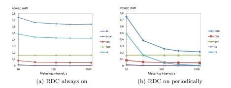
**Fig. 2.** Power consumption at a constrained device, both total and according to modes of operation including CPU active (cpu), low power mode (lpm), transmission (tx), and reception (rx): (a) RDC always on; (b) RDC on periodically. Note that a logarithmic scale is used for the metering interval shown on the x-axis.
