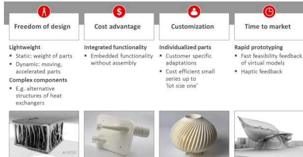
Fig. 3. - Key differentiation criteria for Laser Sintering
