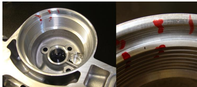
Fig. 11. - Porosity in bed plate at oil filter cartridge (right: enlarged view)
