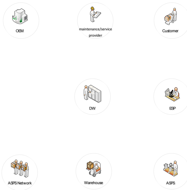
Fig. 7. Key stake holders of an Additive Manufactured Spare Parts logistics
