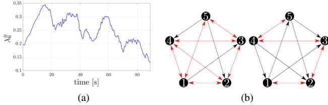
Fig. 6: Behavior of the *unweighted* rigidity eigenvalue  $\lambda_6^B$  (a) and two graph topologies corresponding to the maximum (left,  $|\mathcal{E}| = 17$ ) and minimum (right,  $|\mathcal{E}| = 14$ ) number of edges during the experiment (b).
