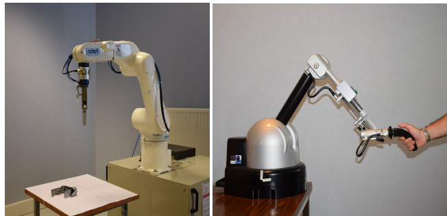
Fig. 1. The experimental setup showing the slave robotic arm on the left and the master haptic arm on the right.
