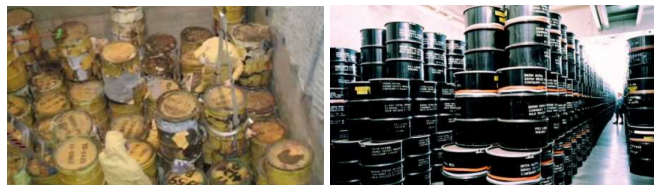
Fig. 1: Left figure: containers with unknown (or partially known) contents and mixed contamination levels that need to be examined, sorted and separated. Right figure: new special storage containers where contaminated waste must be placed.
