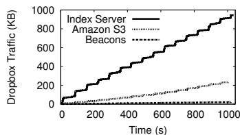
Fig. 4. Dropbox traffic corresponding to rapid, 1 byte appends to a file (5400 RPM HDD).
