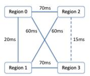
Fig. 8: The experimental topology used to simulate the impact of inter-region link failure, with the failed link (15ms) on the right side.
