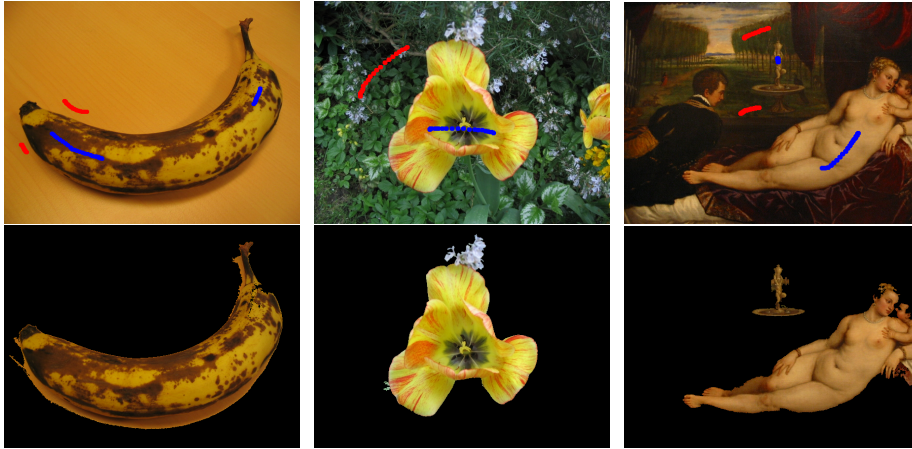
Fig. 9. Interactive segmentation using the CToS. original images with the markers on the top line and the segmentation below.
