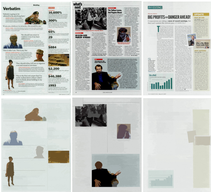
Fig. 11. Simple filtering for document layout detection. Top row: original images; bottom row: results of grain filters.
