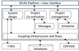
Fig. 1. Architecture of ATLAS prototype
