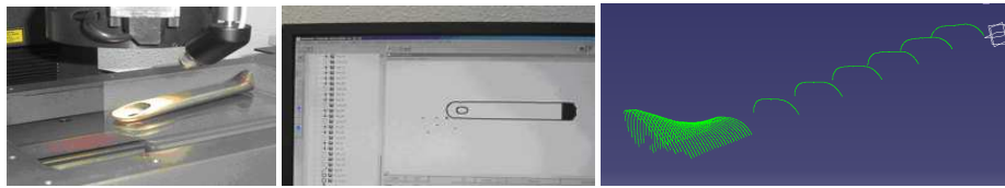
Fig. 4. Optical and laser 3D scanning of final part on CMM, and imported point cloud
