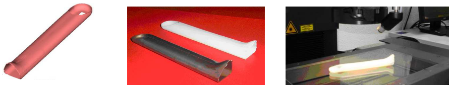
Fig. 9. Rapid prototyping from FE simulation result and control measurement on CMM
