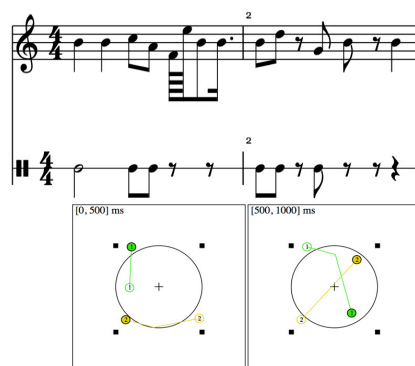
Figure 13: Example score containing spatialization indications exported from a SPAT-SCENE. The cross at the center represents the listener, and the black squares represent the speakers. The colored circles represent the sound sources positions at the beginning (white filling) and at the end (colored filling) of the specified interval. The colored lines represent the actual trajectory between these positions.
