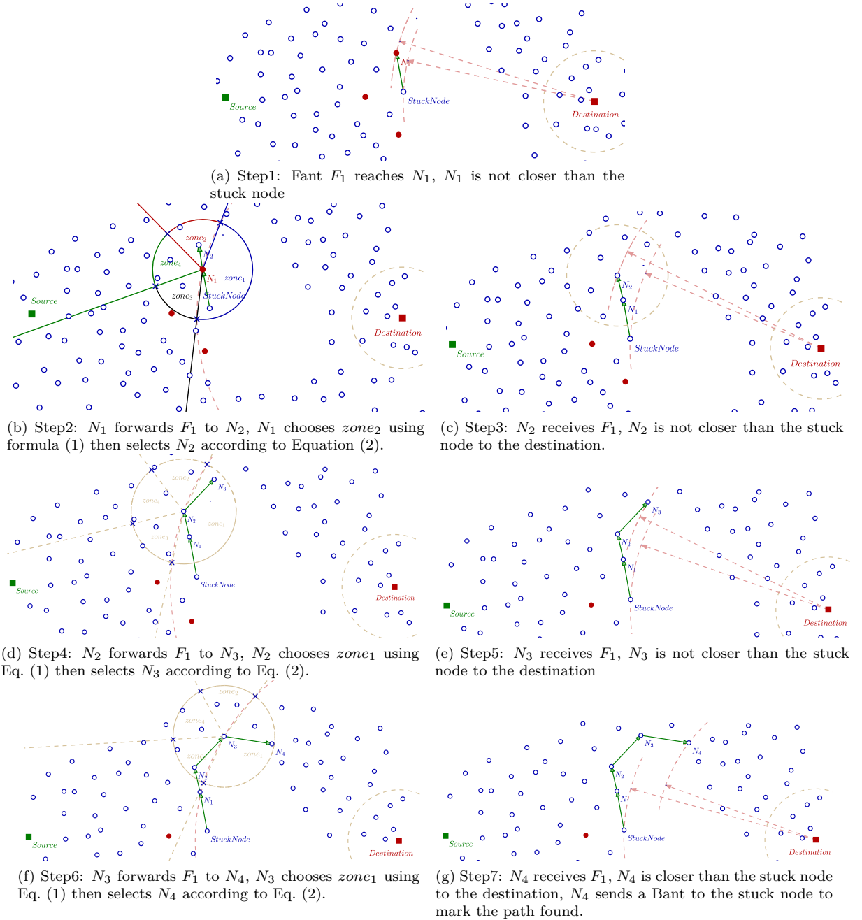
Figure 6: An example of a Fant searching for a path around a void
