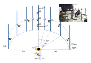
Fig. 2. Environment for capturing real face images.
