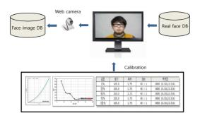
Fig. 4. Procedure for building face image DB.
