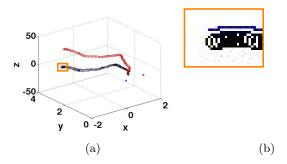
Figure 9: A typical simulated trajectory in presence of disturbance along the z-axis. In blue the true trajectory, in red the trajectory estimated by only integrating the gyroscope and the airspeed measurements and in black the trajectory estimated by the proposed EKF.
