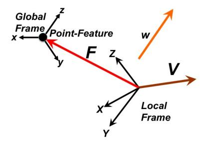
Figure 7: Local and global frame for the considered problem. The z-axis of the latter is aligned with the direction of the disturbance (assumed to be known and constant in time). The speed V is the vehicle speed with respect to the air, which differs from the ground speed because of the disturbance (w).
