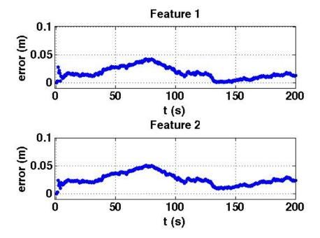
Figure 10: Estimation error on the distance of the two observed point features in absence of the disturbance.
