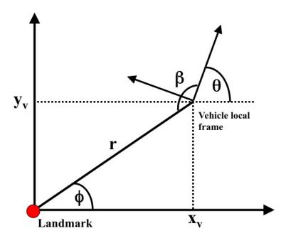
Figure 1: The vehicle state in cartesian and polar coordinates  $([x_v, y_v, \theta]^T)$  and  $[r, \phi, \theta]^T$ , respectively) together with the three considered outputs  $(r, \beta)$  and  $(r, \phi)$ .
