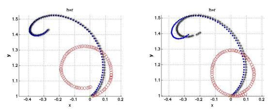
Figure 4: Estimated trajectory in the case when the output is h=r. Dots blue are the ground truth, red circles the estimated trajectory by only using the knowledge of the proprioceptive measurements, black stars the trajectory estimated by our estimator. On the left side is the case when  $\gamma$  is known and on the right side when it is unknown.
