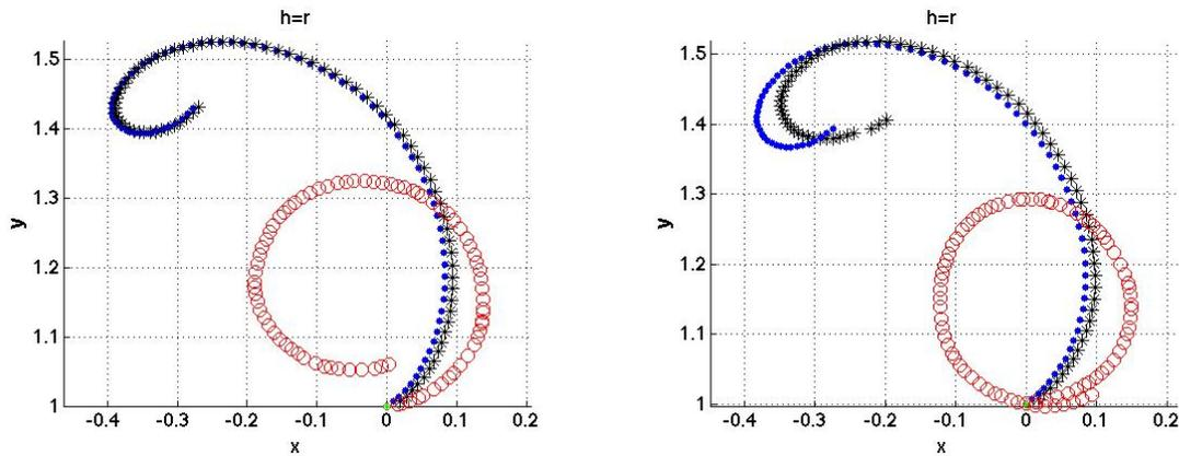
Figure 4: Estimated trajectory in the case when the output is  $h = r$ . Dots blue are the ground truth, red circles the estimated trajectory by only using the knowledge of the proprioceptive measurements, black stars the trajectory estimated by our estimator. On the left side is the case when  $\gamma$  is known and on the right side when it is unknown.
