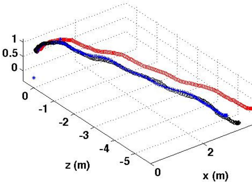
Figure 8: A typical simulated trajectory in absence of disturbance. In blue the true trajectory, in red the trajectory estimated by only integrating the gyroscope and the airspeed measurements and in black the trajectory estimated by the proposed EKF.
