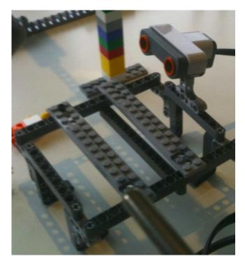
Fig.8. Prototype 3 - The simulated plant table that should hold plant material for obtaining real sensor data
