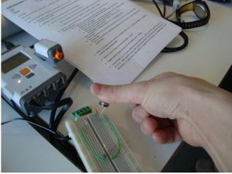
Fig.11. Testing and calibrating the light sensor
