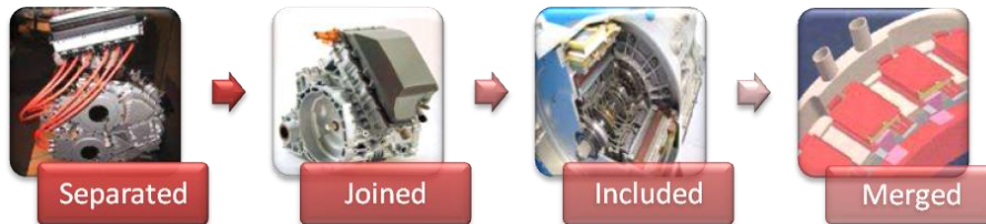
Fig. 1. The different integration levels in mechatronics system design [5]
